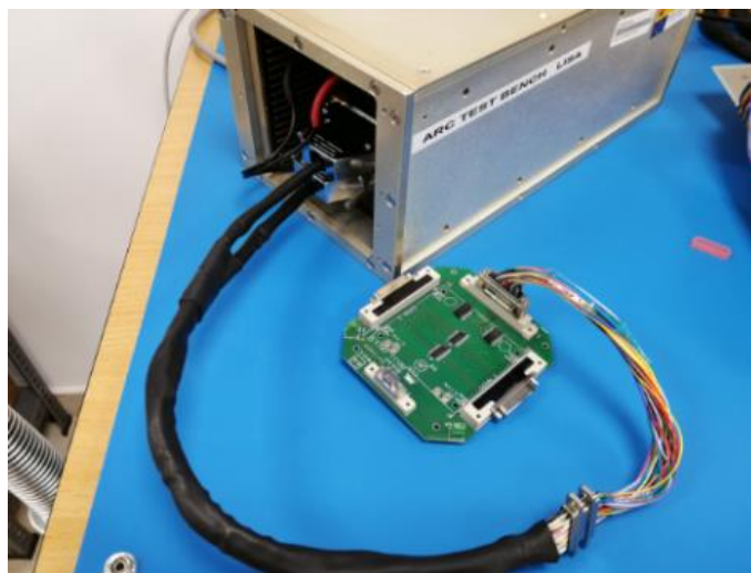
Figure 28: ARCGenIII controller, including wiring and the cryogenic interface of the detector.
