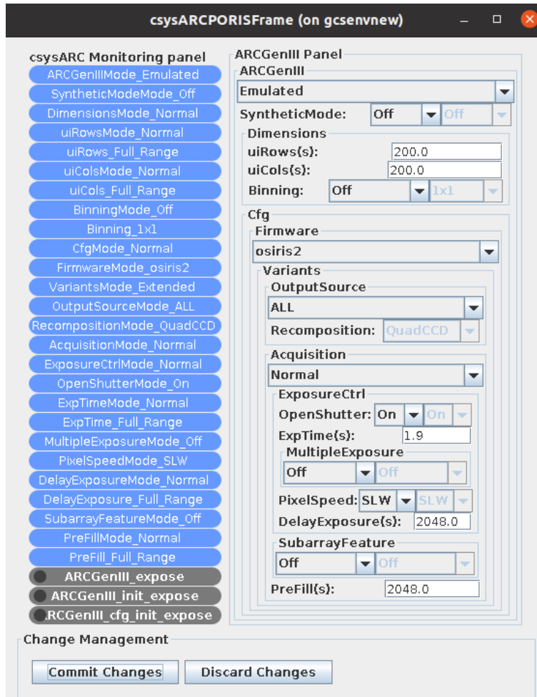
Figure 32: Configuration panel after the user configures the instrument in emulated mode using the 'osiris2' firmware variant and setting the OutputSource to 'ALL'. In the left half of the panel, in blue capsules, the device monitors have appeared shortly after the user has pressed the 'Commit Changes' button.
